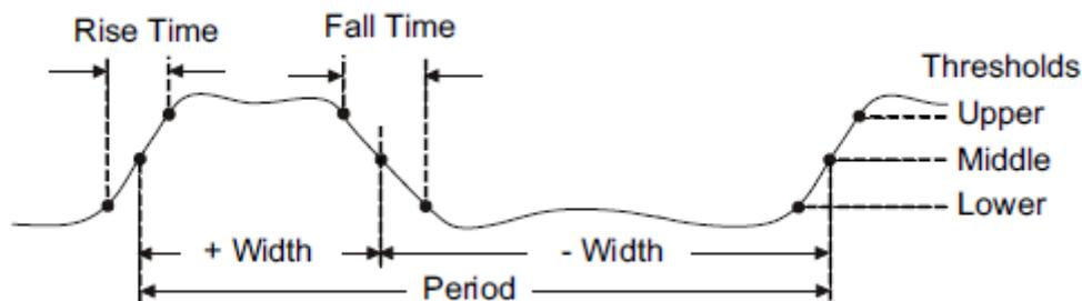
Figure 89 Time Measurements
