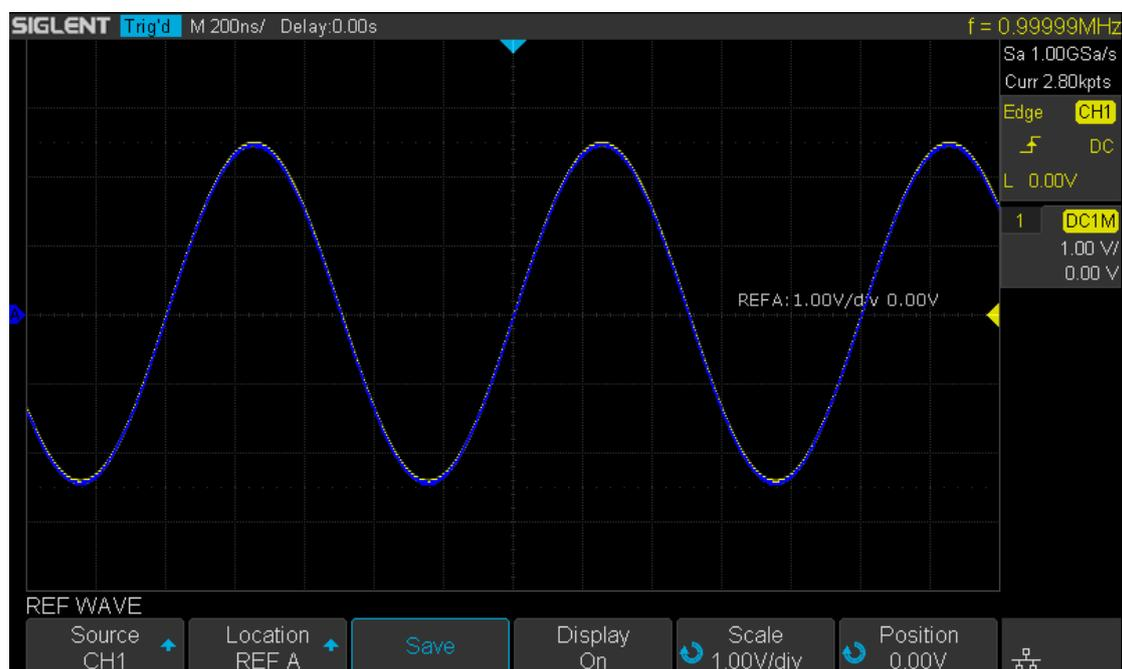
Figure 69 Reference Waveform
