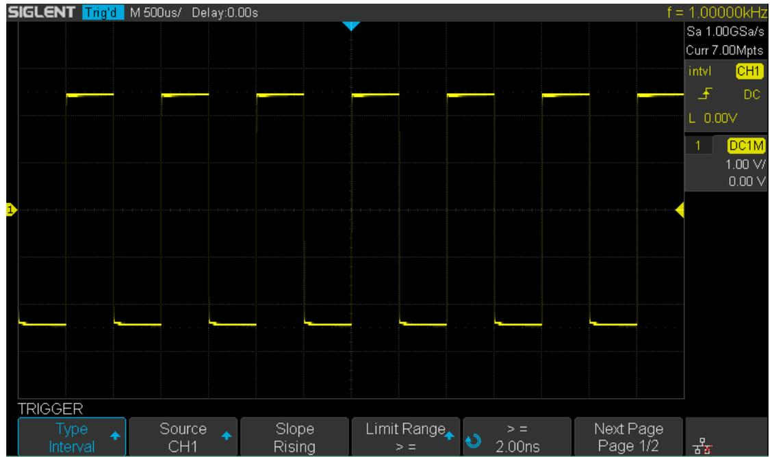
Figure 36 Interval Trigger
