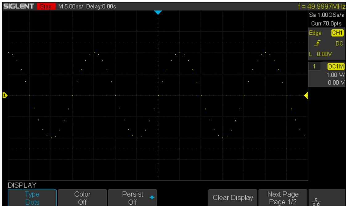
Figure 95 Dots Display
