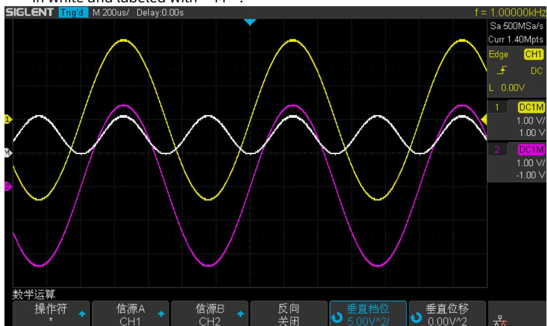
Figure 71 C1\*C2 Waveform
