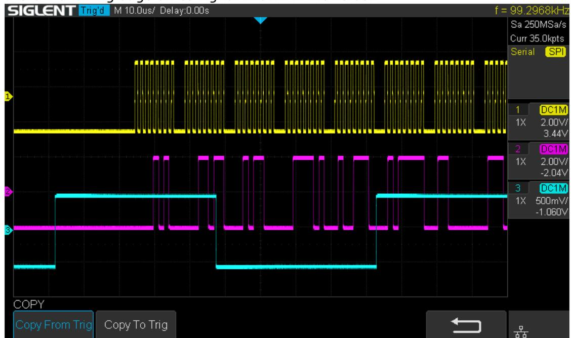
When the CS type is set to Clock Timeout, the clock idle time between frames is  $T_3$ , the clock period is  $T_1$ , then set the timeout to a value between  $T_1$  and  $T_3$ :
