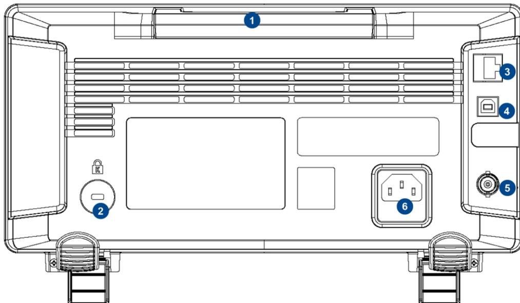
Figure 13 SDS1000X-U Scope Rear panel Overview
