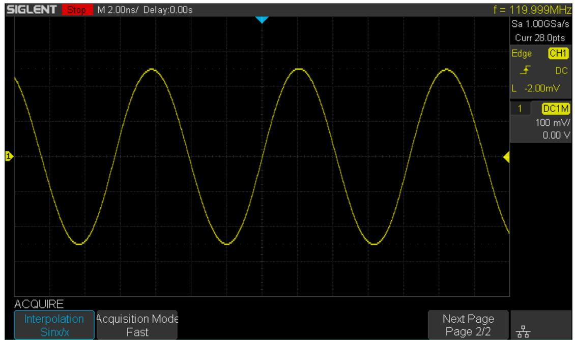
Figure 20 Sinx/x Interpolation
