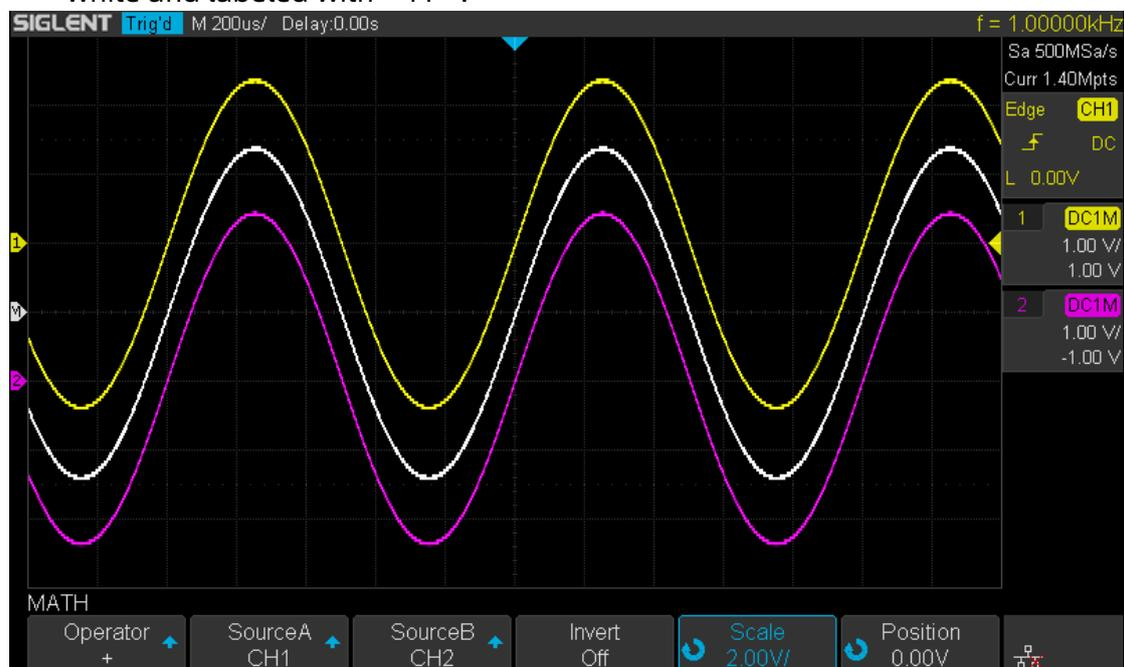
Figure 70 C1+C2 Waveform
