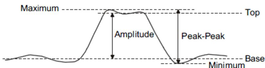
Figure 86 Voltage Measurements
