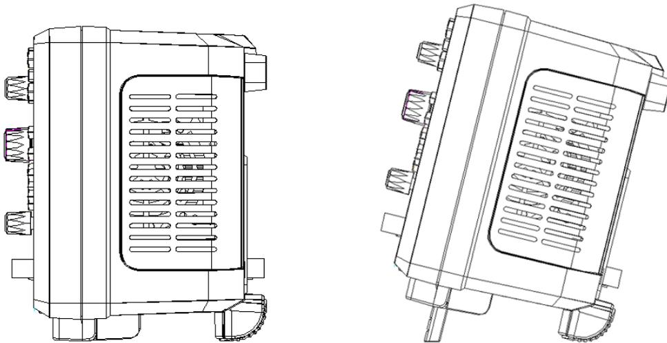
Figure 5 Adjust the Supporting Legs
