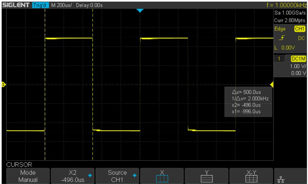
Figure 85 Measure Pulse Width
