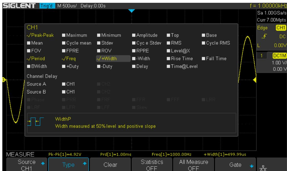
Figure 90 Select the Measurement Parameter
