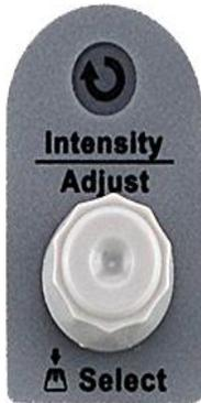
**1. Adjust the waveform intensity.**
