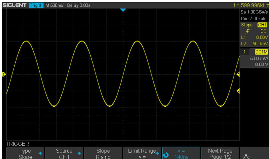
Figure 31 Slope Trigger
