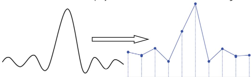
2. **Waveform Confusion:** when the sample rate is lower than twice the actual signal frequency (Nyquist Frequency), the frequency of the waveform rebuilt from the sample data is lower than the actual signal frequency. The most common aliasing is the jitter on fast edge.
