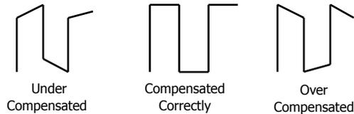
3. Use a nonmetallic driver to adjust the low-frequency compensation adjustment hole on the probe until the waveform changes to be correct as the figure above.
