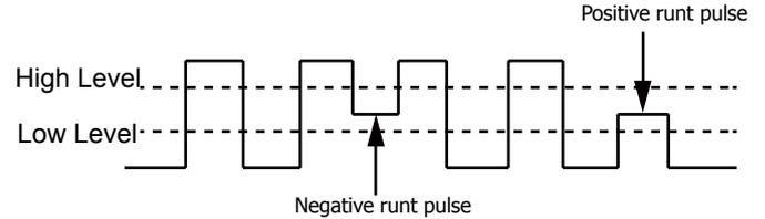
In the figure below, the trigger signal are positive runt pulse.
