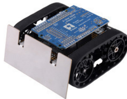
Assembled Zumo Robot for Arduino with an Arduino-compatible A-Star 32U4 Prime LV.
