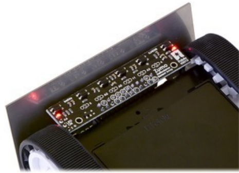
Zumo reflectance sensor array on a Zumo robot, bottom view.
