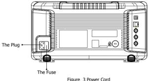
Figure 3 Power Con Connection
