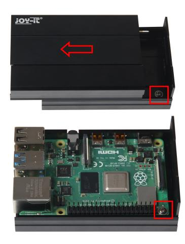
4. Now slide the cover back onto the case and screw tighten the two upper screws again. You now have the choice of placing the GPIO cover on the case or keeping it free.
