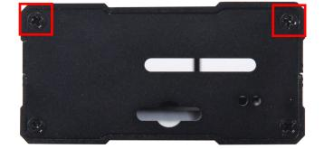
3. The upper part of the case can now be pushed out to the side. Loosen the now visible screw to insert and fix the Raspberry-PI.
