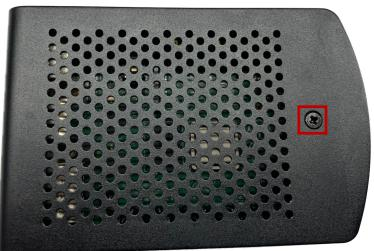
4. Now you can mount the mounting brackets if requierd. These need to be screwed onto the bottom of the case.
