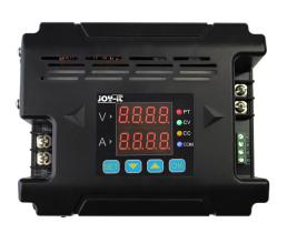
The JT-DPM8624 is a programmable Buck power supply. It has both a constant voltage and a constant current mode. With the RS-485 interface, it is possible to manage any setting comfortably via your PC with a free software.
