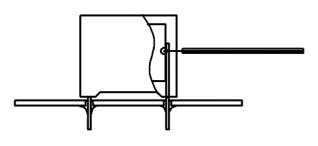
The temperature is monitored inside the capacitor.
