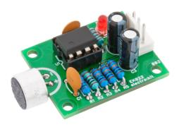
external resistor should be mounted in series with the output. The amplifier is preset for 100x gain, but the gain can be modified by changing the feedback resistor (R3). The gain is calculated using the formula G=R2/R3 (1k/100k = 100x gain). The OP-amplifier used is a low voltage, low noise type and can be powered from 3V up to 12V.
