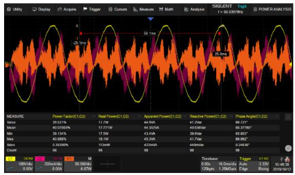
Siglent SDS5000X Power Analysis and Bode Plot function are very convenient and a great time saving option for power circuit engineers.
