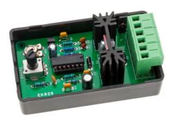
used for setting the maximum pulse time. To trim the generator, turn VR1 fully clockwise. Slowly turn VR2 until the output is fully on (100% pulse width). If the trimmer is turned too far, the output will revert to 50% pulsewidth. The kit can be powered using the same voltage as the motor or a separate supply if the motor voltage is higher than 15V. To use a common supply, JMP1 must be bridged. Please observe that the maximum voltage on V+ is 15V!
