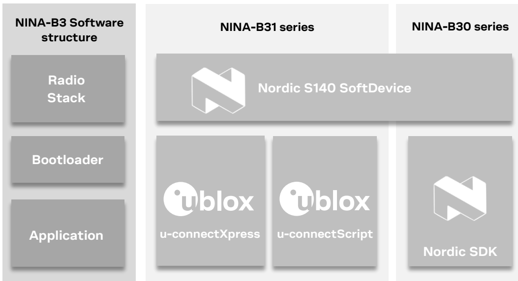
Figure 2: NINA-B3 software structure and available software options
