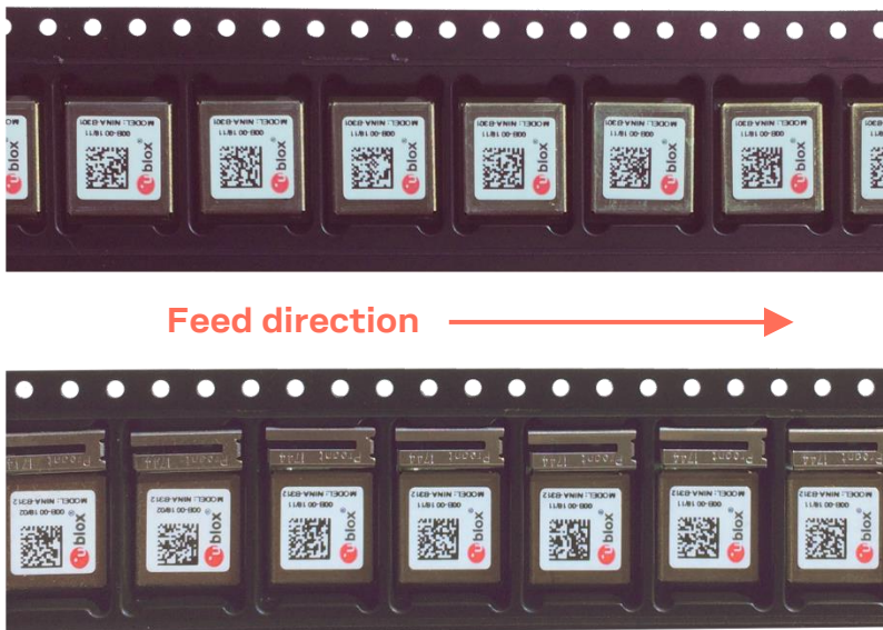
Figure 16: Orientation of NINA-B3 modules on tape.
