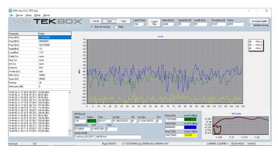
The main graph displays the measured field strength of the observed transmitters on the y- Axis and the index number of the corresponding measurement on the X-axis.
