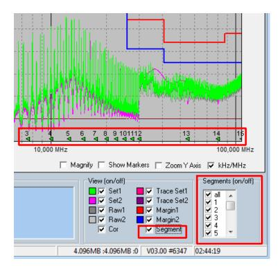
As Quasi-Peak measurements take much time, an alternative, time saving measurement method is recommended.
