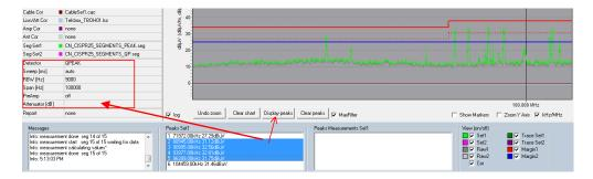
The software will then re-measure, using the selected peaks as center frequency and using the detector, sweep time, RBW, Span and PreAmp settings defined in the control box. This feature is a short cut to make
