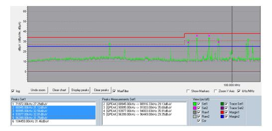
The Peaks Measurements box then displays the results of the fast quasi peak measurement. In addition, the graph shows a cross at the respective frequency and level.
