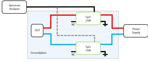
Example: conducted emission pre-compliance test of an automotive LED driver Using 2 pcs Tekbox TBOH01 5µH LISN
