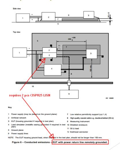
Applicable Tekbox LISN for conducted measurements at mains terminals: 1 x TBOH01 or 2 x TBOH01
