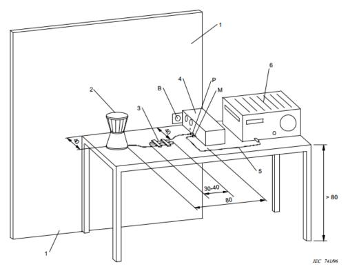
Measurement set up example taken from CISPR 16:
