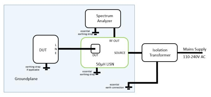
The DUT shall be isolated and elevated from the groundplane. The spectrum analyzer shall measure conducted emissions on both line and neutral.
