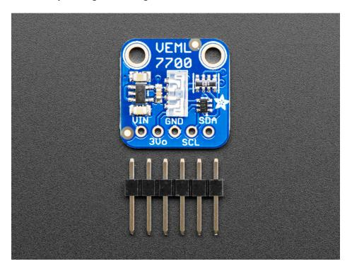
Interfacing is easy - this sensor uses plain, universal I2C. We put this sensor on a breakout board with a 3.3V regulator and logic level shifter so you can use it with 3.3V or 5V power/logic microcontrollers. We have written libraries for Arduino (https://adafru.it/EoE) (C/C++) as well as CircuitPython (Python 3) (https://adafru.it/EoF) so you can use this sensor with just about any kind of device, even a Raspberry Pi!
