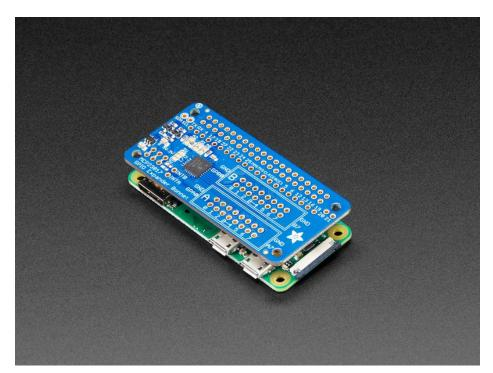
When used as an input, you can set up a pull-up resistor so buttons and switches don't need extra resistors - just wire the pin to one side and ground to the other! There's interrupt capabilities on the chip, and two IRQ pins (INTA and INTB) you can solder a wire to, if you want to have a quick way of telling if any of the GPIO's changed.
