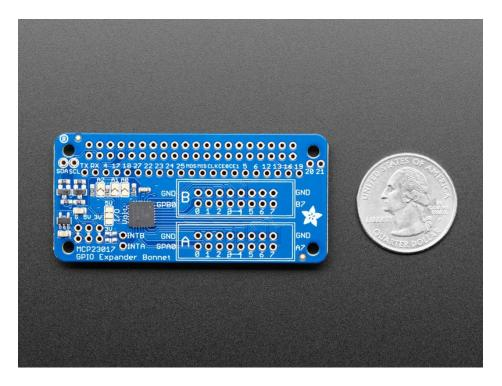
By soldering closed the address select jumpers, you can change the address from 0x20 up to 0x27. So, if you wanted to, you could have up to 8 bonnets for 128 total GPIO.
