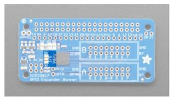
This Bonnet defaults to using 5V. There is a jumper to swap between 3V and 5V. If you want to change it to 3V, you can cut the trace between the top two pads, and solder the bottom two pads.
