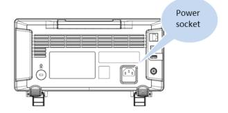
Figure 4 Connect the Power Supply
