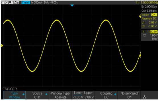
Figure 28 Absolute Window Trigger
