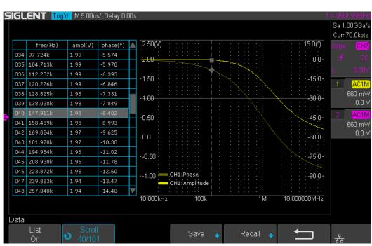
2) Press **Save** softkey (**Recall** softkey) to enable the bode plot save (recall) function. The details of save (recall) see the chapter "Save and Recall".
