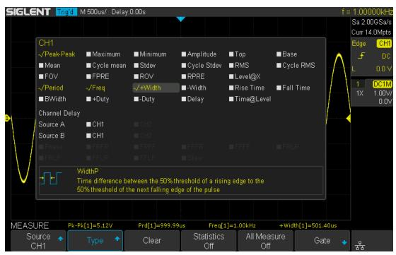
Figure 66 Select the Measurement Parameter
