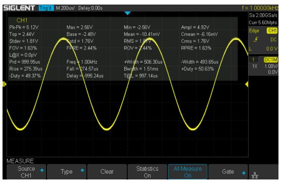
Figure 68 All Parameters Measurement
