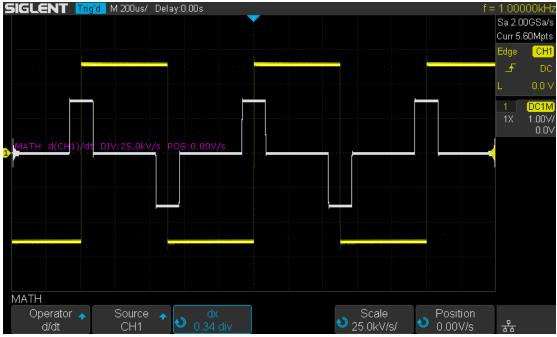
Figure 57 Differential Function Operation
