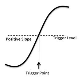
You can adjust the trigger level for a selected analog channel by turning the **Trigger Level Knob**.
