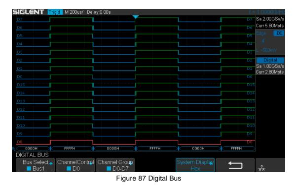
• The Sampling rate of digital channels is displayed at the right of the display.
