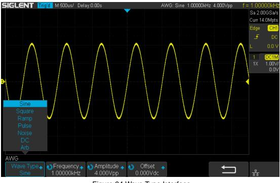
Figure 94 Wave Type Interface
