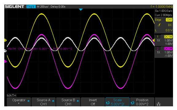
Figure 55 CH1\*CH1 Waveform
