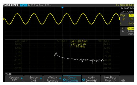
Figure 56 FFT Waveform in Split Mode
