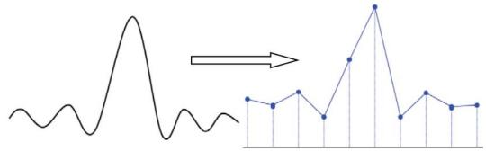
2. Waveform Confusion: When the sample rate is lower than twice the actual signal frequency (Nyquist Frequency), the frequency of the waveform rebuilt from the sample data is lower than the actual signal frequency. The most common aliasing effect is the
