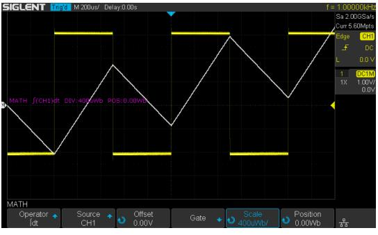
Figure 59 Integral with Offset
