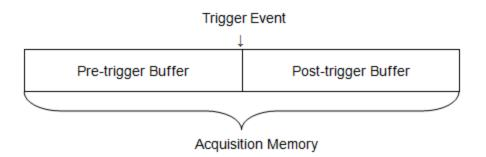
Trigger settings should be based on the features of the input signal, thus you need to have some knowledge of the signal under test to quickly capture the desired waveform.
