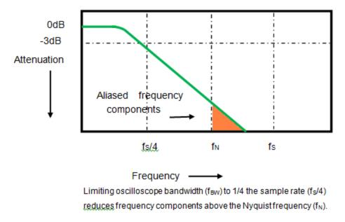
So, in practice, an oscilloscope's sample rate should be four or more times its bandwidth:  $f_s = 4fBW$ . This way, there is less aliasing, and aliased frequency components have a greater amount of attenuation.
