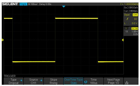
Figure 32 State Dropout Trigger
