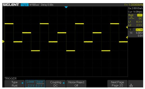
Figure 33 Runt Trigger
