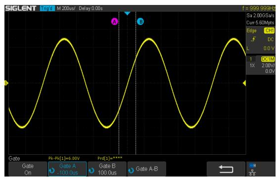
Figure 69 Gate measurement
