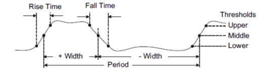
Figure 65 Time Measurements
