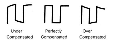
3. Use a nonmetallic driver to adjust the low-frequency compensation adjustment hole on the probe until the waveform displayed is as the "Perfectly compensated" in the figure above.
