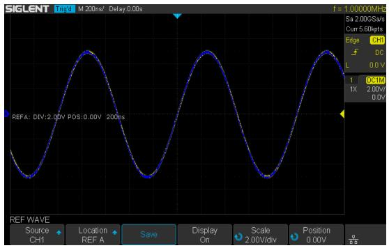
Figure 53 Reference Waveform
