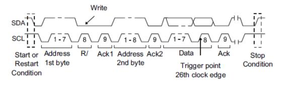
• Data Length — When SDA data's length is equal to the value of Byte Length and address's length is the same as set value, the oscilloscope will be triggered. Byte length is in the range of 1 to 12 bits.
