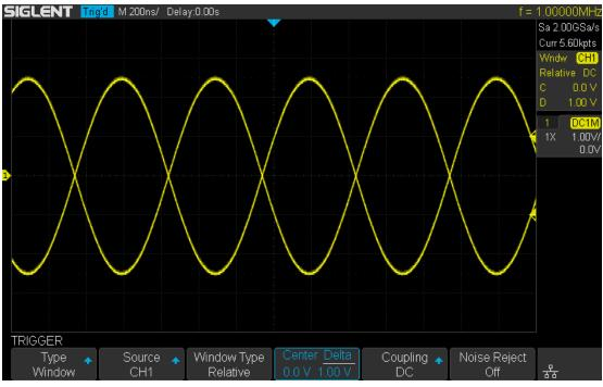
Figure 29 Relative Window Trigger
