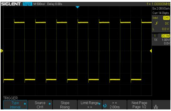
Figure 30 Interval Trigger
