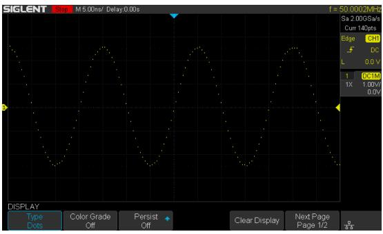
Figure 75 Dots Display
