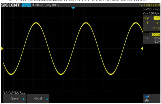
5. Press the **Press To Save** softkey to enter the SAVE/RECALL file system.
