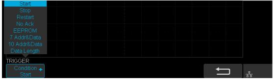
Figure 37 I2C TRIGGER Menu
