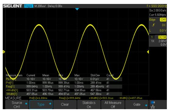
Figure 67 Adding the Measurement
