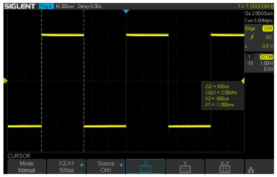
Figure 61 Measure Pulse Width
