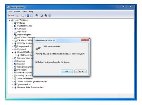
Click OK and the libusb driver should be completely uninstalled for the device.
