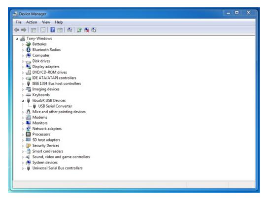
If you see the libusbK node and USB serial device, move on to the next step to install libftdi.
