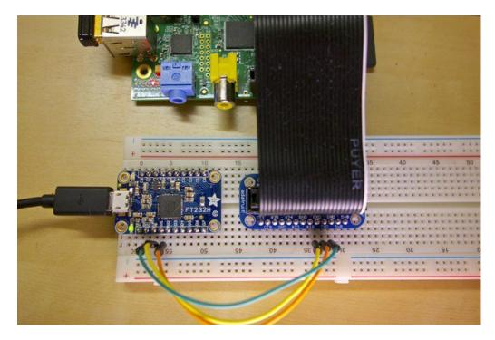
Use PuTTY or screen to open the FT232H serial port at 115200 baud and you'll be accessing the Raspberry Pi's serial port!
