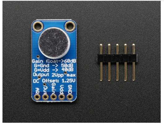
Assembly is really easy, you can use straight or 'right-angle' style headers to attach to the PCB. We'll be using the plain straight headers included
