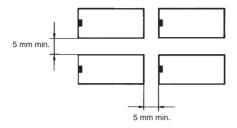
The above minimum mounting space is necessary due to mutual thermal interference generated by the relays. This restriction may be ignored, however, depending on the operating conditions of the relays. Consult OMRON for details.
