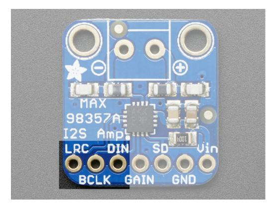
Three pins are used to receive audio data. These can be 3.3-5V logic
