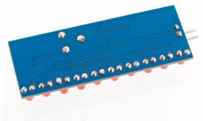
Trim all the leads and make a final visual inspection to make sure there are no bad solder joints, bridges, debris or other faults in the assembly. Connect a power supply to the pin header (3 – 12VDC) and watch in awe as the LEDs light up and flow like water in the spring.
