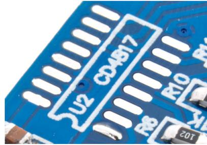
Place and align the IC using tweezers. Make sure both rows of the IC align up with the pads. Alignment must be correct before soldering the rest of the pins!
