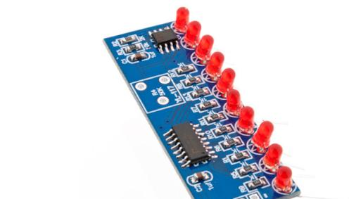
Flip the board and notice the poor alignment. Melt the solder and press down on each LED to align them properly. When they are all in a straight line, solder the other lead.
