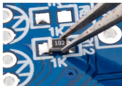
Melt the solder on the pre-tinned pad to fixate the component. As long as only one pad is attached, you can make adjustments by melting the solder again and again until a perfect alignment has been achieved.
