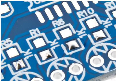
Start by pre-tinning one pad for each of the passive components. Only a small amount of solder is required.
