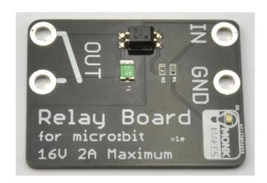
The MonkMakes Relay for micro:bit is a solid-state (no moving parts) relay that allows an output of a micro:bit to turn things on and off.
