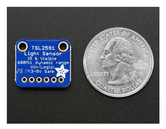
This sensor is much like the TSL2561 but with a wider range (and the interface code is different). This sensor has a massive 600,000,000:1 dynamic range! Unlike the TSL2561 you cannot change the I2C address either, so keep that in mind.
