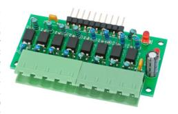
four outputs are non-inverting. All inputs are rated for voltages between 3.3V and 15V. For use with lower or higher signal levels, the current limiting resistors for the LEDs in the optocouplers must be replaced with a lower or higher resistance value to keep the maximum allowed current below 30mA.
