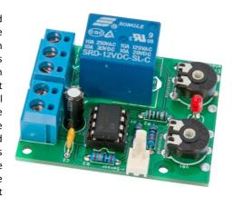
the relay from entering an unstable state, a hysteresis is implemented. The hysteresis is set by the resistor R3. To reduce or completely remove the hysteresis, change the resistor to a higher value or omit the resistor. The connector for the sensor is a Molex KK 2.54mm. A mating connector with wires is sold separately (part.no. 41002820).
