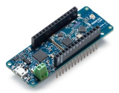
**Arduino**® **MKR FOX 1200** has been designed to offer a practical and cost effective solution for makers seeking to add SigFox connectivity to their projects with minimal previous experience in networking. It is based on the Atmel SAMD21 and a ATA8520 SigFox module.
