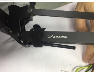
Note: Because there is no need to use the silicon tube for suction cup, we could use the velcro to fix the tube with the upper arm.
