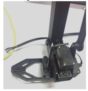
Step 2: Plug the wire of gripper
