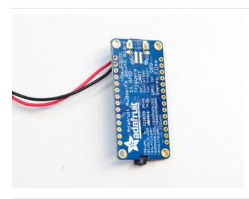
For most battery packs the red wire is the positive wire, connect that to Vin. The black wire is ground, connect that to GND.
