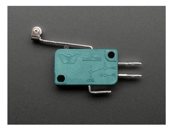
In this case, we connect the COM (common) pin to ground, then the normally-closed to pin #10 and the normally open to pin #0
