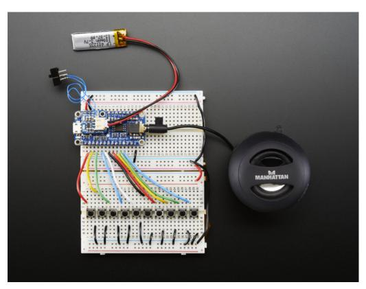
And a version with built in class D stereo amplifier, you can have  $2 \times 2.2W$  of output audio power, driving 4 or 8 ohm speakers
