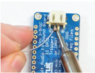
Solder all four pads - two mechanicals on the side, and two power coming out the end.
