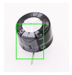
Note: Capacitor has positive and negative point. The mark in the above picture is negative point. Electrolytic capacitor has a white line. The footer is comparatively shorter.
