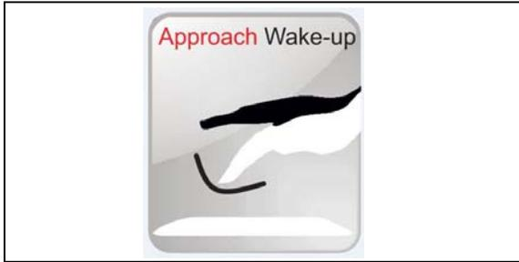
Approach Detection is an embedded power-saving feature of Microchip’s Colibri Suite. It sends MGC3X30 to Sleep mode and scans periodically the sensing area to detect the presence of a human hand.
