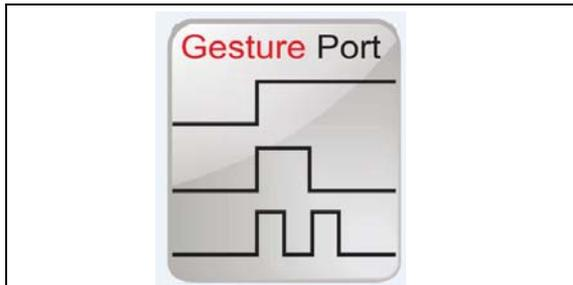
The Gesture Port enables a flexible mapping of Colibri Suite feature events to certain output signals at dedicated pins of the MGC3X30. The individual feature events can be mapped to one of five EIO Pins and trigger a variety of signal changes (Permanent high, Permanent low, Toggle, Pulse (100 ms), High Active, Low Active). The Gesture Port simplifies and enhances embedded system integration. It enables host-free integration based on EIOs.
