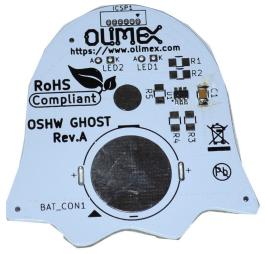
The colophony flux in the solder wire do a little messy look but do not worry, at the end you can use Isopropile or Ethyl alcohol with soft fabric to clean the flux residues. Even if not clean they are harmless for the board, just will not look pretty as the picture above :)
