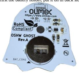
Then flip the PCB and solder the legs which are seen on front side:
