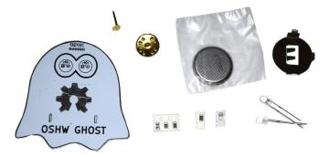
What you see is white printed circuit board, metal clip and pin which will allow you to attach this board to your cloths, battery and metal battery holder, 3 resistors one capacitor and two high intensity green LEDs with 3 mm diameter.
