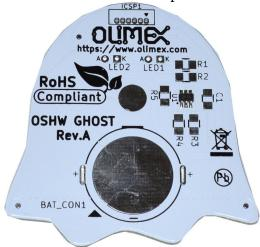
This is done intentionally for two reasons, first it's hard to solder for novices, second to pre-program it we use the ICSP1 connector on top, to program this PIC microcontroller in bulk requires special adapter we do not have:)
