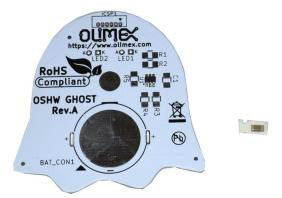
You must peel the transparent tape and take off the capacitor then to solder it to C1 pads on the board like on this picture.
