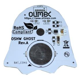
Then you need for find three resistors in paper tape, they are marked 121 = 120 or 120 Ohms! These must be soldered to R1, R2, and R4 locations:
