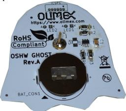
We are almost done! Now put the LEDs on their places, but note that they have POLARITY so you have to put them with the shorter leg inside the square pad (marked as K) and longer led in the circle pad (marked as A).
