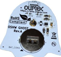
Now is time to attach the battery, again be careful as battery has polarity the + must be pointing UP as
