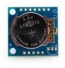
This battery powered clock allows you to keep reasonably accurate time even when your Arduino is powered off. It's very useful in data logging and other time sensitive applications.
