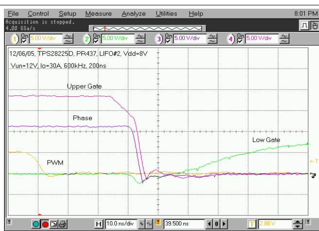
Figure 40. Phase Falling-Edge Switching Waveforms (10 ns/div) of the Power State in Figure 25
