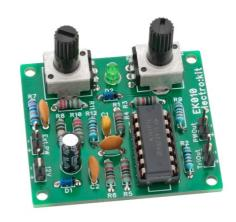
potentiometer with 1Mohm. If lower or higher frequencies are required, replace the timing capacitor C1 with a smaller or larger value. The outputs are protected with 1kohm resistors, which also sets the output impedance. This kit alone is not suited for driving motors or LEDs directly, but when combined with kit EK010b, it can be used for driving loads up to 24V 5A. To use this kit for audio purposes, a series capacitor should be mounted on the outputs to eliminate the DC offset.
