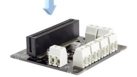
Inserting a BBC micro:bit: To use the motor driver board the BBC micro:bit should be inserted firmly into the connector as shown left.
