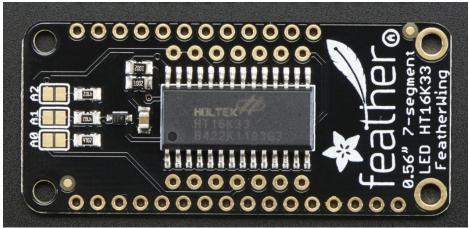
The 7-segment backpack makes it really easy to add a 4-digit numeric display with decimal points and even 'second colon dots' for making a clock
