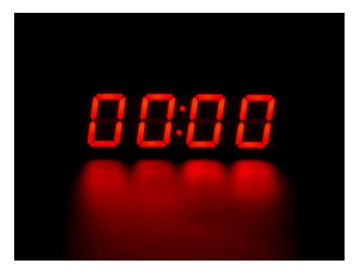
The LEDs themselves do not connect to the Feather. Instead, a matrix driver chip (HT16K33) does the multiplexing for you. The Feather simply sends i2c commands to the chip to tell it what LEDs to light up and it is handled for you. This takes a lot of the work and pin-requirements off the Feather. Since it uses only I2C for control, it works with any Feather and can share the I2C pins for other sensors or displays.
