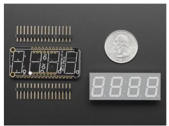
When you buy a pack from Adafruit, it comes with the fully tested and assembled backpack as well as a 7-segment display in one of the colors we provide (say, red, yellow, blue or green). You'll need to solder the matrix onto the backpack but it's an easy task.
