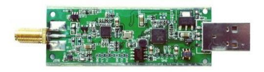
The RTL-SDR Blog V3 is an improved RTL-SDR dongle. RTL-SDR dongles were originally designed for DVB-T HDTV reception, but they were found by hardware hackers to be useful as a general purpose SDR. The standard dongles are okay for DVB-T reception, but are just barely suitable for SDR users/experimenters. The RTL-SDR Blog V3 was redesigned with SDR user needs in mind, instead of DVB-T HDTV users who typically have more relaxed requirements.
