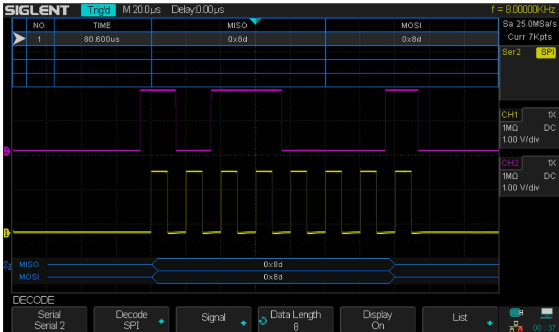
Figure 46 SPI Decode
