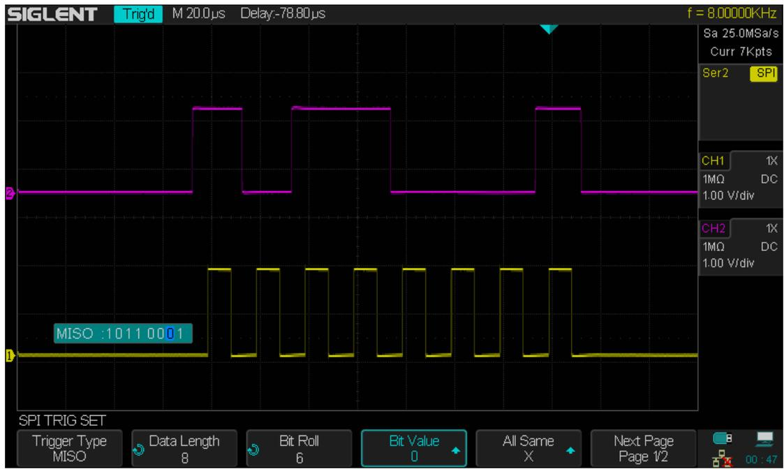
Figure 44 SPI Trigger
