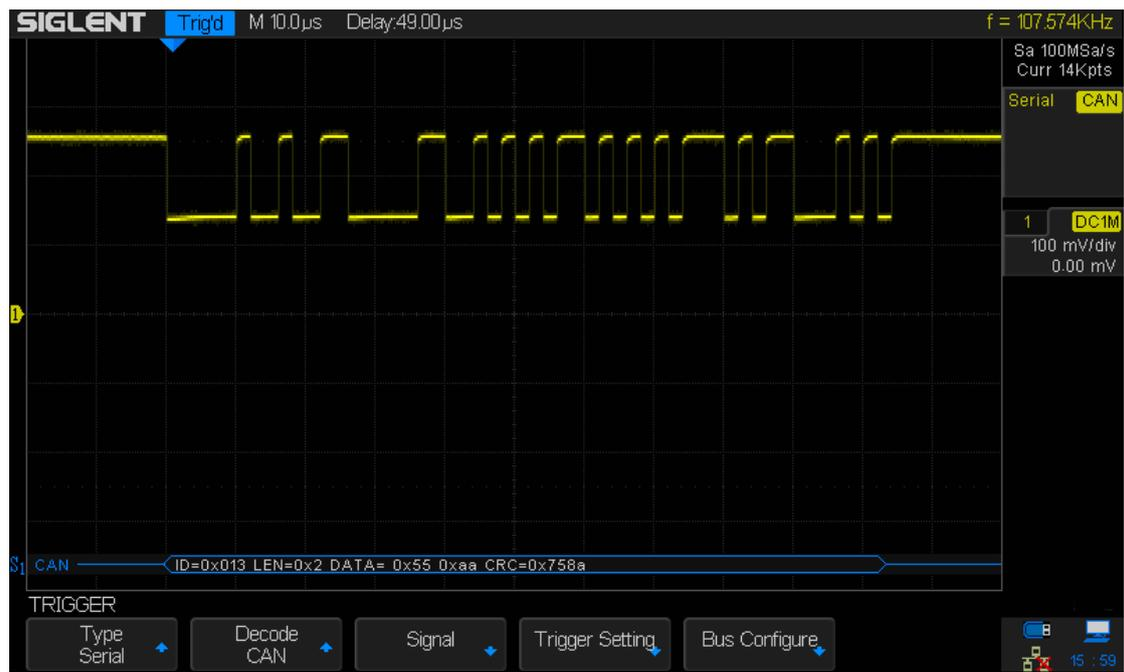
Figure 54 CAN Trigger
