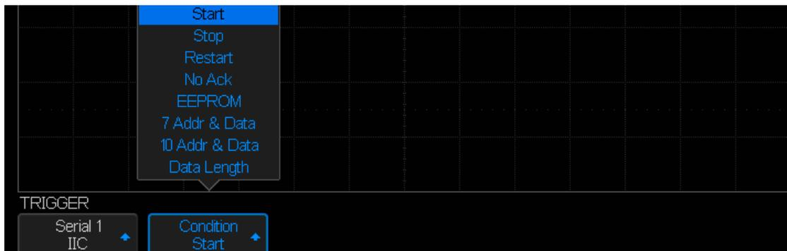
Figure 35 IIC TRIGGER Menu
