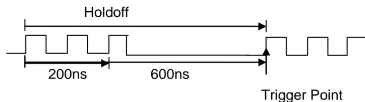
The correct holdoff setting is typically slightly less than one repetition of the waveform. Set the holdoff to this time to generate a unique trigger point for a repetitive waveform. Only edge trigger and serial trigger have holdoff option. The holdoff time of the oscilloscope is adjustable from 100ns to 1.5s.
