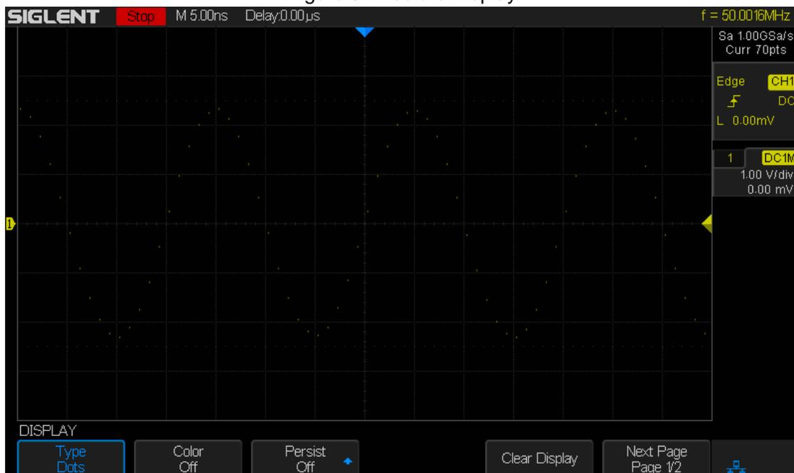
Figure 83 Dots Display
