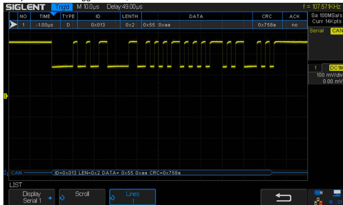
Figure 55 CAN Decode
