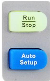
**Auto Setup** : press this key to enable the waveform auto setting function. The oscilloscope will automatically adjust the vertical scale, horizontal time base and trigger mode according to the input signal to realize optimum waveform display.
