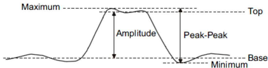
Figure 75 Voltage Measurements
