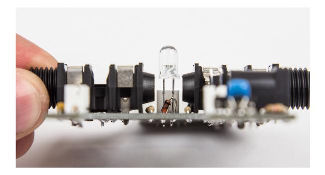
17. 5 mm white LED: LD3 (do a diode test with a multimeter to find the white LED)
