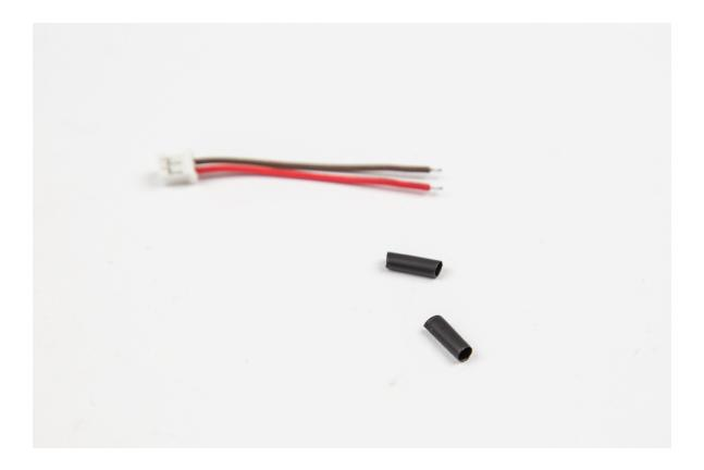
36. Solder the wires to the footswitch as shown below. **Do not forget the shrinktube pieces and note the colors.**
