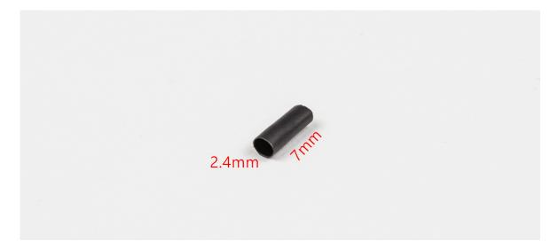
C. Slide both the 3 mm white LED and the 3 mm photo transistor in the shrink tube as shown below. No need to actually shrink the tube. This will act as the lightbridge.
