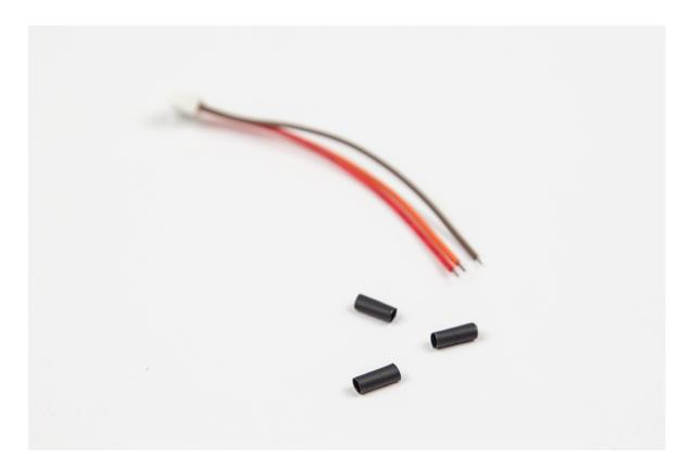
48. Solder the wires to the B100K potentiometer as shown below. **Do not forget the shrinktube pieces and note the colors.**
