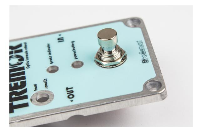
27. Install the selector switch as shown in the images below.
