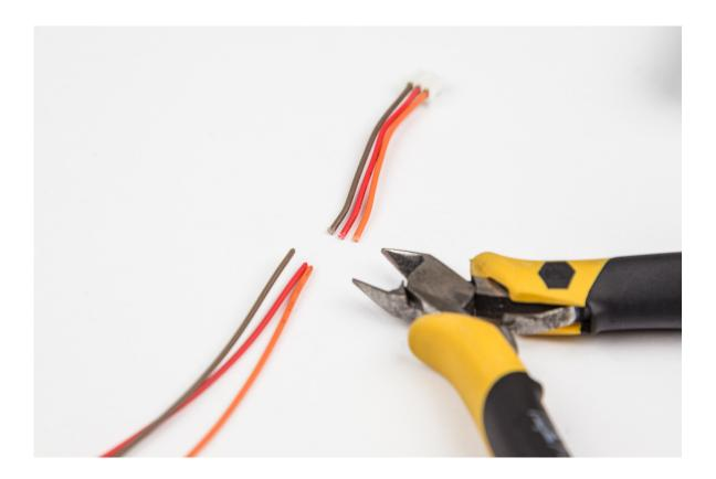
42. Strip and tin the wires of both connectors.
