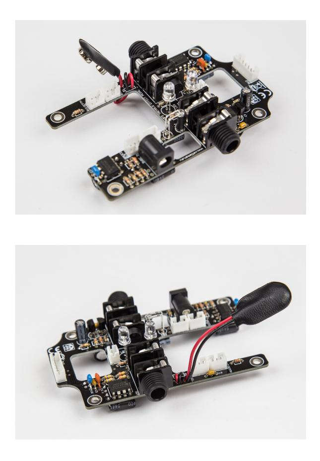
23. Slide 4,5 cm of the biggest shrinktube over the connector. When no battery is used in the pedal this cover should always be used.
