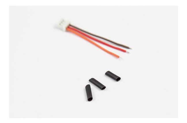
40. Solder the wires to the selector switch as shown below. **Do not forget the shrinktube pieces and note the colors.**
