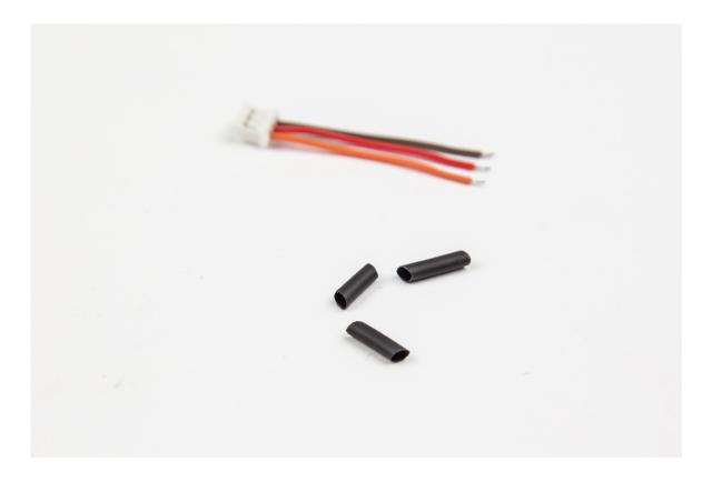
44. Solder the wires to the 500K and the B10K potentiometer as shown below. Do not forget the shrinktube pieces and note the colors.
