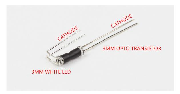
D. Place and solder this assembly in LD2 and P1. Note the orientation of both cathode pins!
