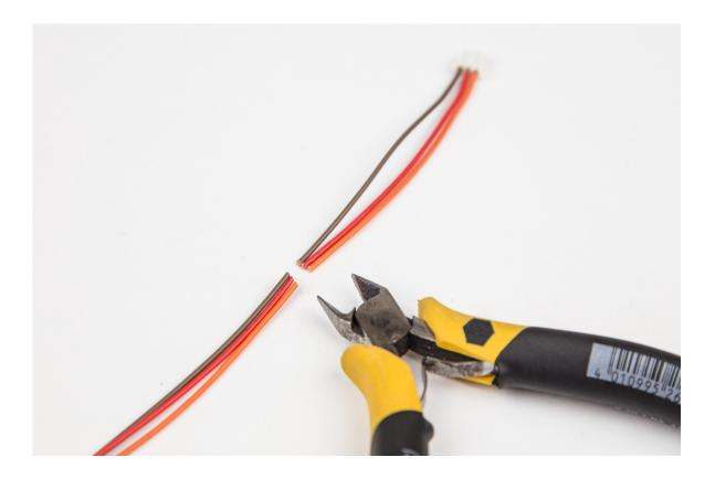
46. Strip and tin the wires of the connector.
