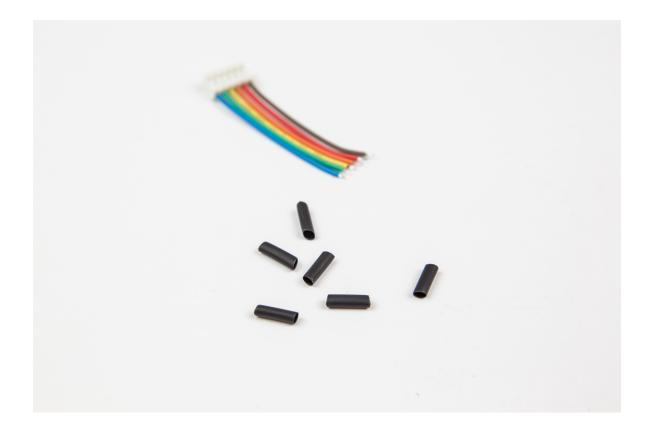
32. Solder the wires to the footswitch as shown below. **Do not forget the shrinktube pieces and note the colors.**
