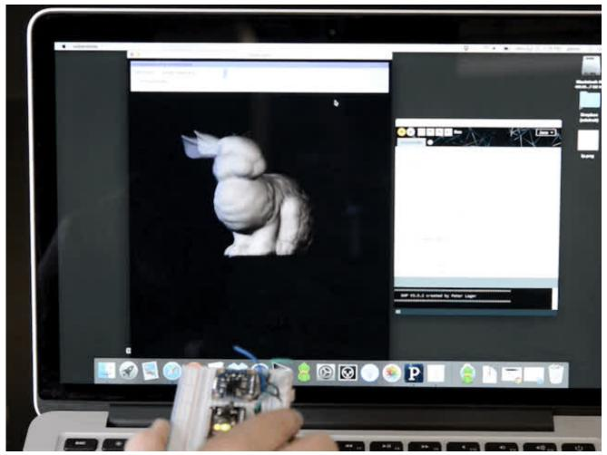
Also notice in the upper right corner of the dialog box at the top that the calibration of each sensor is displayed. It's important to calibrate the BNO055 sensor so that the most accurate readings are retrieved. Each sensor on the board has a separate calibration status from 0 (uncalibrated) up to 3 (fully calibrated). Check out the video and information from this guide for how to best calibrate the BNO055 sensor (http://adafru.it/kA1).
