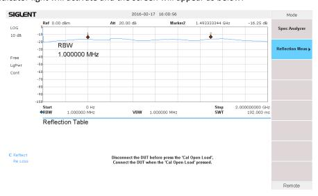
2) In the Reflection Measurement mode the user can modify certain spectrum analyzer parameters such as **Frequency**, **Amplitude**, and **BW**, in those related menus.
