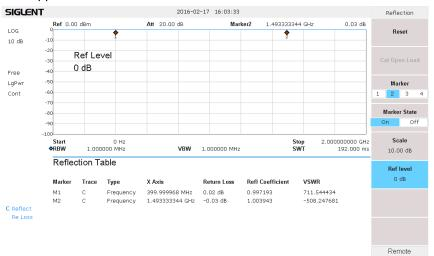
4) Connect the device under test with the DUT terminal of the reflection bridge. The cables or adapters between the DUT and bridge should as short as possible, in order to reduce extra mismatches. The resulting display appears as below. The trace on the screen is the return loss of the device under test.
