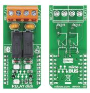
RELAY click<sup>™</sup> is an add-on board in mikroBUS<sup>TM</sup> form factor. It's a compact and easy solution for adding RELAY to your design. It features two G6D1AASI-5DC power PCB relay modules as well as two screw terminals. RELAY click<sup>™</sup> communicates with target board microcontroller via mikroBUS<sup>TM</sup> PWM (RL1) and CS (RL2) pins. The board is designed to use 5V power supply only. LED diode (Green) indicates the presence of power supply.
