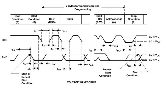
Figure 1. I<sup>2</sup>C Interface Load Circuit and Voltage Waveforms
