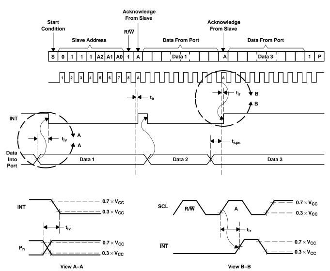
Figure 2. Interrupt Voltage Waveforms
