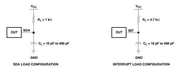
Figure 4. Load Circuits
