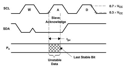
Figure 3. I<sup>2</sup>C Write Voltage Waveforms
