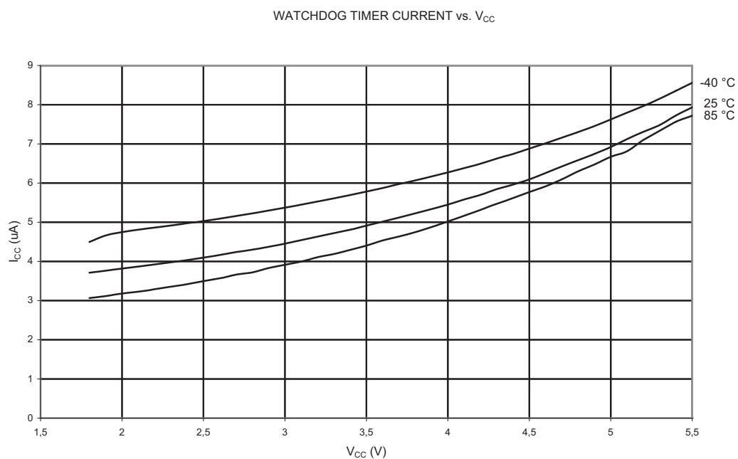
Figure 17-50. Watchdog Timer Current vs. V_{CC}
