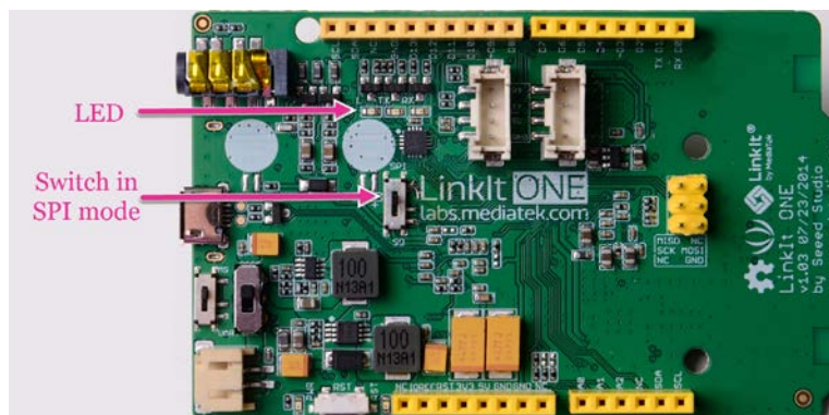
Figure 12 The LED on the LinkIt ONE board
