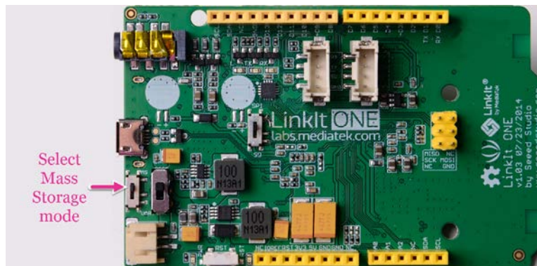
Figure 13 LinkIt ONE in mass storage mode
