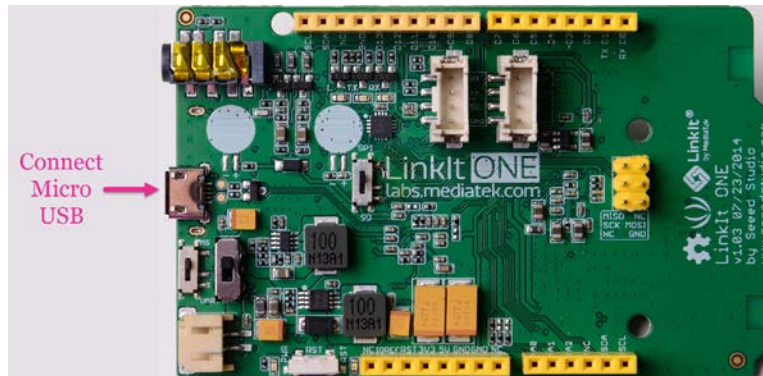
Figure 8 LinkIt ONE Micro USB connector
