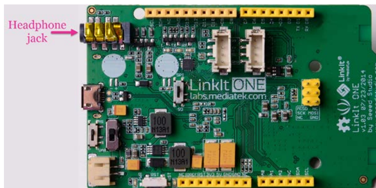
Figure 20 The headphone jack on LinkIt ONE
