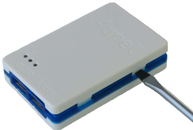
Figure 2-13. Opening the Atmel-ICE (2)
