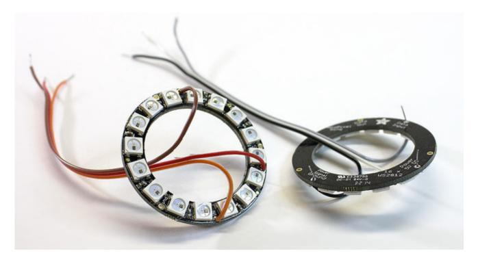
Notice how the wires are inserted from the front, then *soldered on the back* of the ring. **Do it this way if you're new to soldering**...it's much easier. It *can* work the other way too...insert from back, solder on front...but the component tolerances are *extremely* tight
