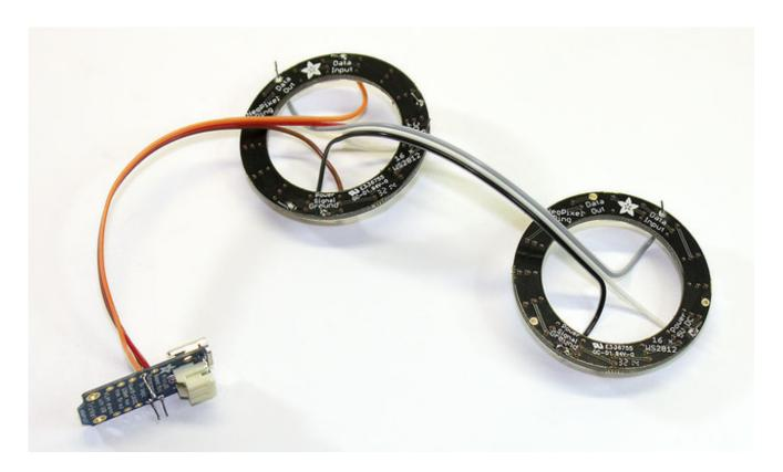
If possible, try to align the rings so they're pointed nearly the same direction (use a landmark like the Adafruit logo for reference). This is not required, but it's a little easier to program animation effects when both rings have the same orientation.
