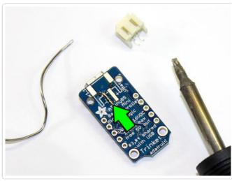
Start by "tinning" one of the JST pads on the back of the Trinket...heat the pad and apply solder so the whole surface is covered.
