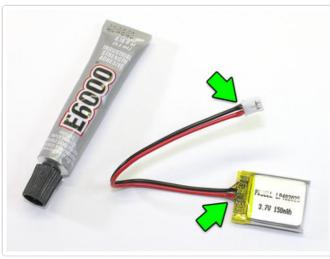
This step is **optional** but **recommended:** if you have some 5-minute epoxy or craft adhesive such as E6000, add a small bead at the base of each wire where it meets the board...and *especially* on the LiPoly battery and JST connector. This creates a *strain relief*, so wires aren't likely to break off when flexed. On the NeoPixel rings, it helps the wires sit flat.
