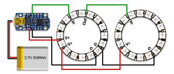
Solder one end of the 3-wire cables to the IN, V+ and G points on the two NeoPixel rings. There are *two* V+ and *two* G holes on each ring...either one is fine, they're connected.
