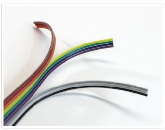
Next, peel away two sets of three wires each from the included bit of ribbon cable. (If you're building your own custom goggles, you can just use separate pieces of wire for this, it's all good.)
