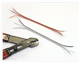
Separate the wires by about **1 inch** at **both ends**, strip away a little insulation and give the wires a twist to prevent fraying. Optionally *tinning* the wire ends makes them a little more manageable...heat each one with a soldering iron and melt just a tiny bit of solder into the strands.
