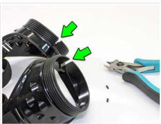
The costume goggles have slots near the nose piece, bridged by a tiny bit of plastic. If these are clipped away, then all the electronics can be slid in place from the front. You might also **cut the slots just a little wider** so they don't gouge the wires.
