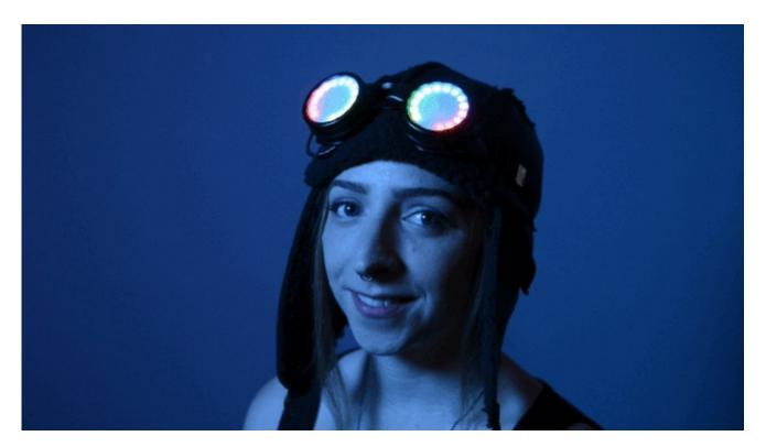
Adafruit NeoPixel LED rings fit perfectly inside the eyecups of most 50mm round goggles — a very common size. It's almost as if these rings were *made* with this project in mind!
