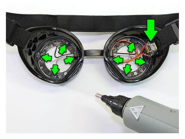
**PRO TIP:** if you used hot glue and need to remove the rings later, dip a Q-Tip in rubbing alcohol, touch it to the edge of each blob of glue and allow it to soak in for a few seconds. This doesn't dissolve the glue; it seeps between the two parts and cleanly breaks the bond. The glue should peel away with little effort. Science!
