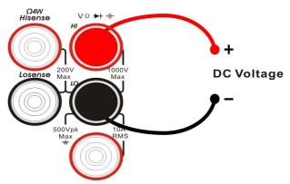
Diagram 2-5 Sketch Map for Measuring DC Voltage
