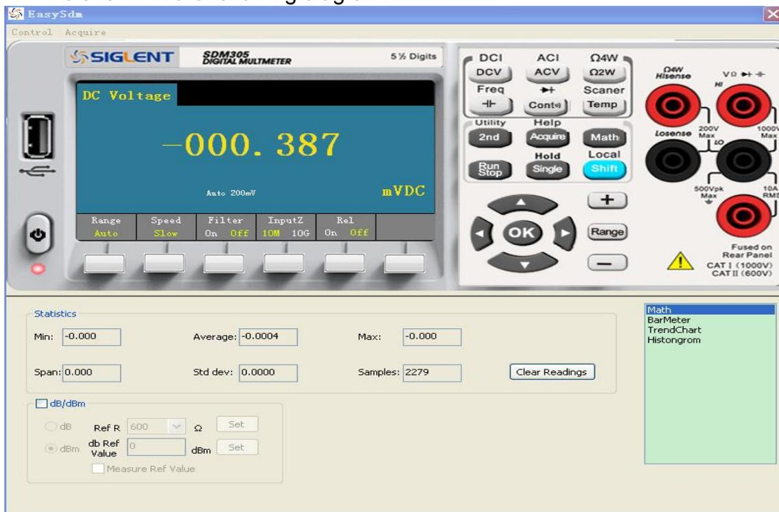
Diagram 3- 19 The Main Interface of EasySDM
