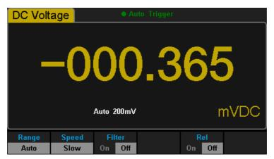
Diagram 2-4 DC Voltage Measurement Interface
