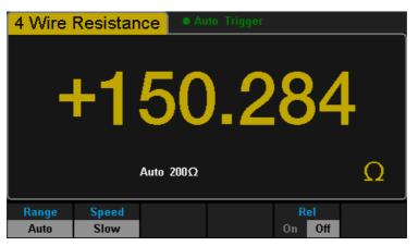
Diagram 2-15 4-Wire Resistance Measurement Interface
