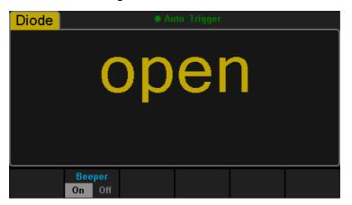
Diagram 2-25 Diode Test Interface
