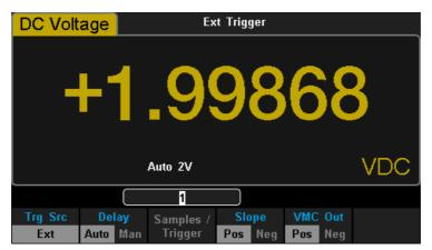
Diagram 2-54 Setting interface of Ext Trigger
