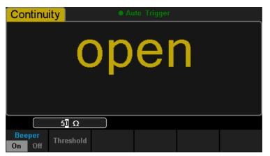
Diagram 2-36 Set Up the Short-circuit Resistance
