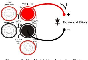
Diagram 2-26 Sketch Map for testing Diode
