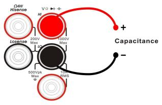
Diagram 2-18 Sketch Map for Measuring Capacitance
