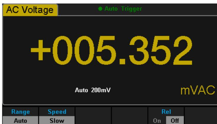
Diagram 2- 8 AC Voltage Measurement Interface
