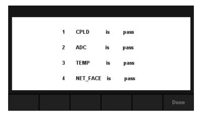
Diagram 2-49 Chip Test Interface
