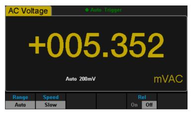
Diagram 2-8 AC Voltage Measurement Interface
