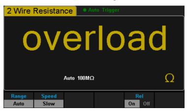
Diagram 2-13 2-Wire Resistance Measurement Interface
