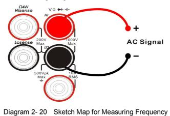
3. Choose a proper voltage range according to the measured circuit.
