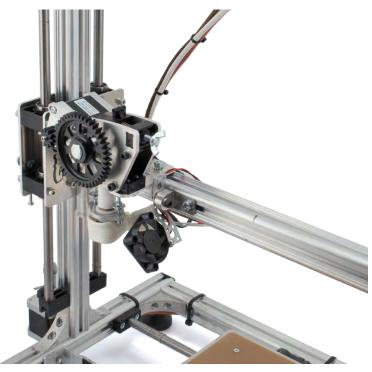
In this way the nozzle of the extruder will be sufficiently separated from the work surface remaining locked to the structure. Place, in a hole of the bracket, an M5 screw (indicated by the red arrow) which will be screwed into the M5 nut previously inserted in the arm.
